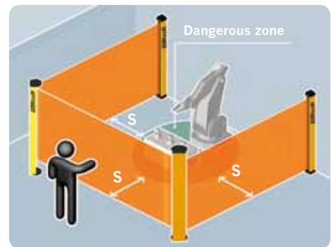
Three-side protection using deflection mirrors
